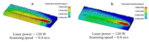
Figure 2. The temperature field and melt pools shape during L-PBF process
