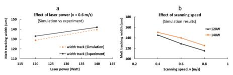
**Figure 4.** The effect of process parameters on melting track width; (a) The effect of laser power (b) the effect of scanning speed
