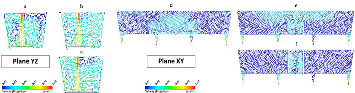
Fig. 5. Velocity flow field on the plane YZ of (a) bare tundish (b) tundish with dam and (c) tundish with baffle; Velocity flow field on the plane XY of (d) bare tundish (e) tundish with dam and (f) tundish with baffle.
