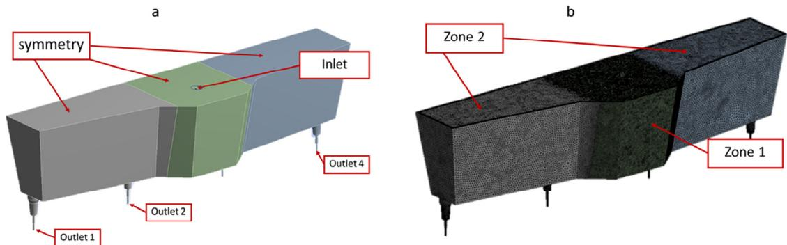
Fig. 3. (a) Geometry and boundary conditions of the 4-strand tundish model with 3 opened outlets; (b) Two zones with different mesh resolution.
