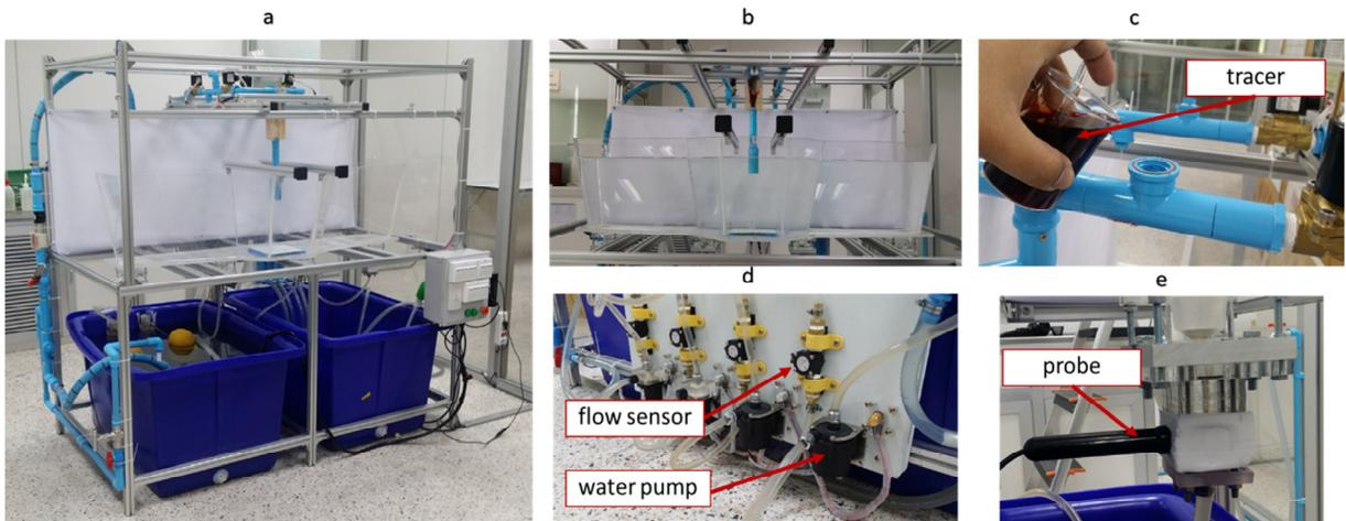
Fig. 4. Experimental setup of (a), (b) the physical water model of multi-strand tundish, (c) tracer, (d) flow sensor and water pump, (e) tracer measured probe.
