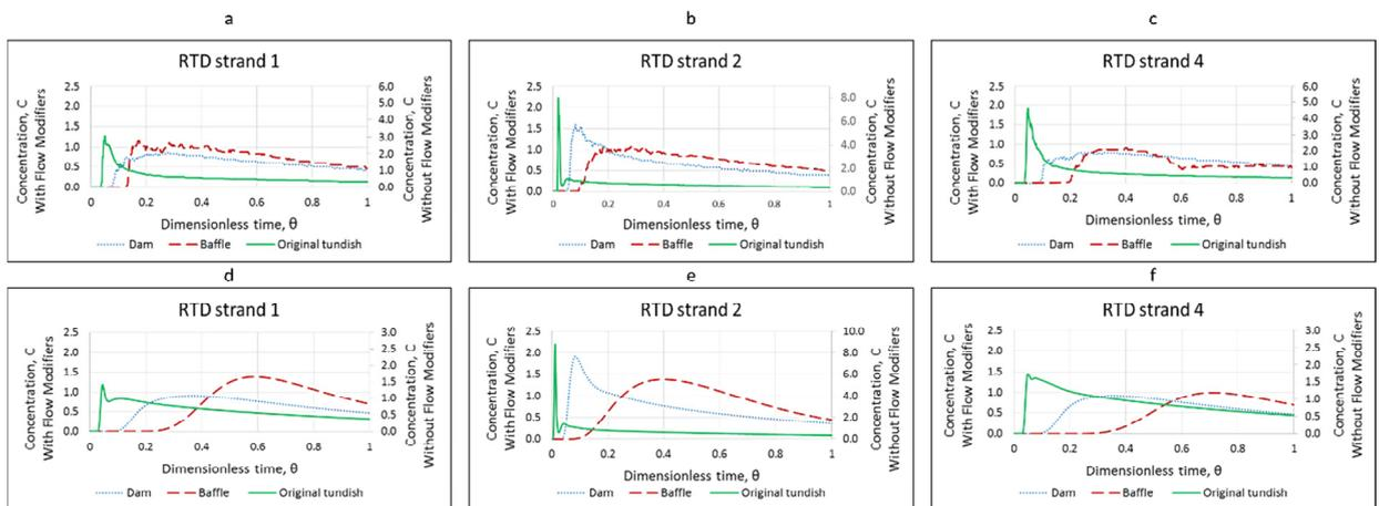
Fig. 8. RTD curves from the CFD simulations from (a) outlet-1, (b) outlet-2, (c) outlet-3; The experiment results from the physical water model at (d) outlet-1, (e) outlet-2, (f) outlet-3.
