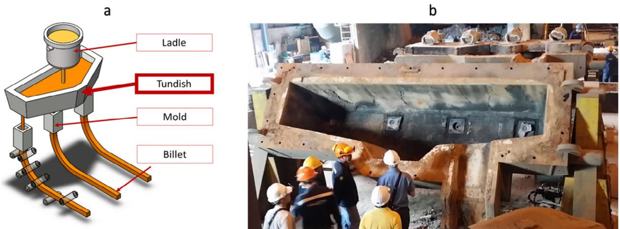
Fig. 1. (a) Diagram of continuous casting process. (b) The 4-strand tundish at Millcon Steel PLC, Thailand.
