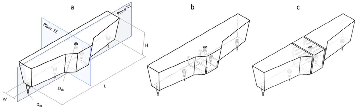
Fig. 2. Geometry of the tundish model with and without flow modifiers: (a) bare tundish, (b) tundish with dam and (c) tundish with baffle.
