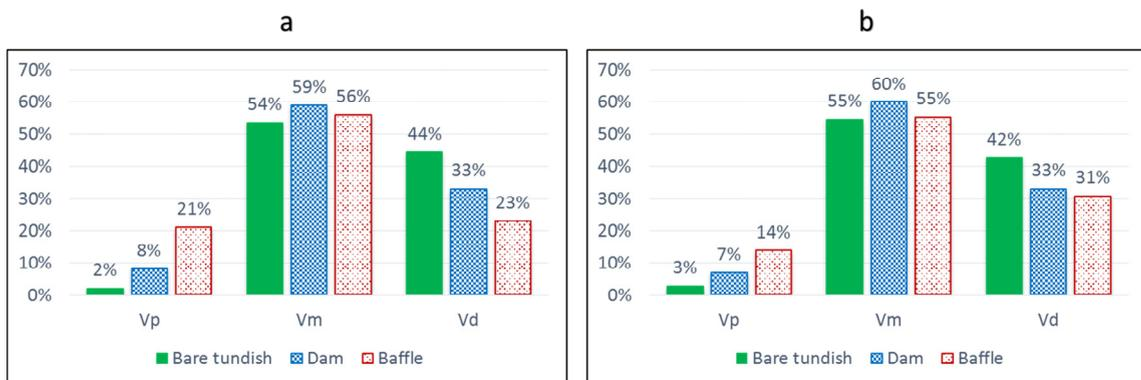
Fig. 9. Volume fraction of the flow in all tundish models obtained from (a) CFD simulation, (b) the physical water model.
