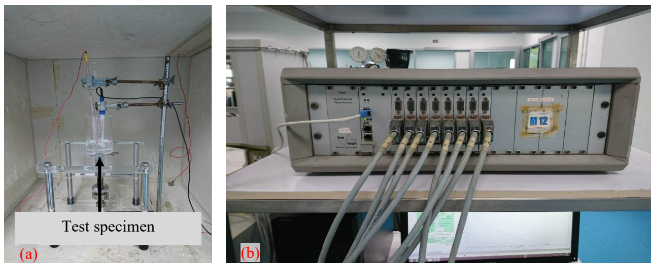
Fig. 2 (a) Self-invented corrosion cell, (b) Biologic science instruments VMP2 multichannel potentiostat.
